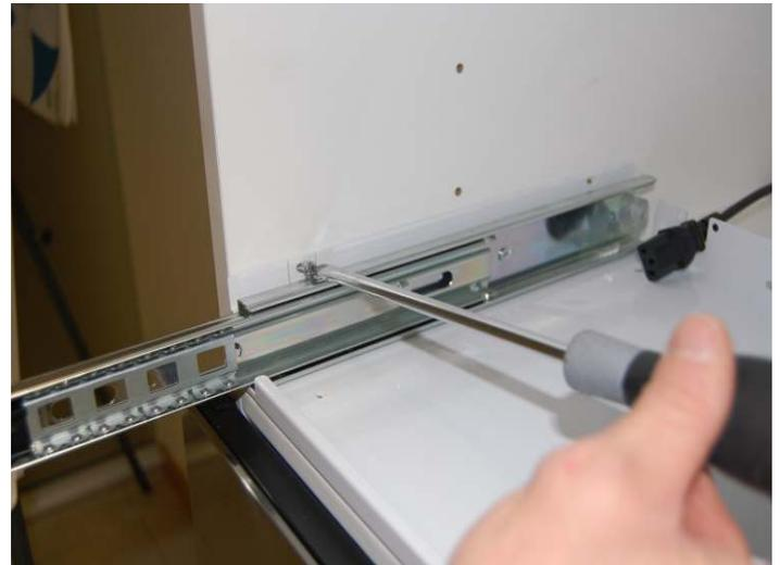
3) Screw the base to the sides (using the x4 screws provided)
