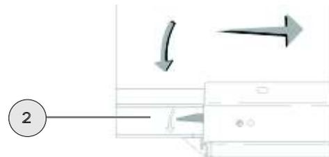
6) If you have to pull out the machine, lift the drawer and pull out.
