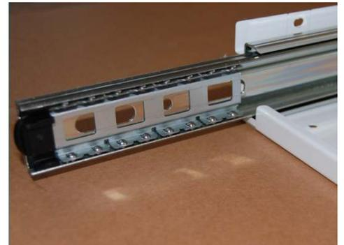
4) Before mounting the unit to the sliding rails, ensure that the bars with the sliding ball bearings are positioned at the front of the rail as shown in the image below. Failure to do this may result in damage to the sliding rails.
